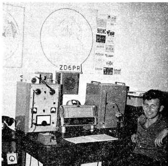
ZD6PR (ex-G3IRQ) in Zomba, Nyasaland, has a Labgear LG300 transmitter, an Eddystone receiver and a Mosley TA33 Jr. aerial.
